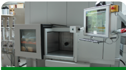
Machine de projection APS
